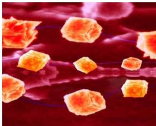
Caption: This image, taken with a scanning electron microscope and digitally colorized and enhanced, shows a new precise biosensor for detecting blood glucose and other biological molecules using hollow structures called single-wall carbon nanotubes anchored to gold-coated "nanocubes." The device resembles a tiny cube-shaped tetherball anchored to electronic circuitry by a nanotube about 25,000 times thinner than a human hair.
