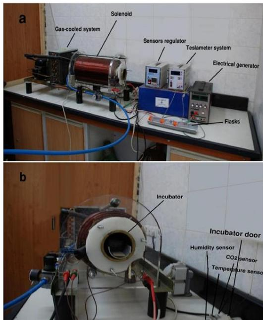
**Fig.. 2 Photograph showing the apparatus used to generate static magnetic field (a) the whole body of the system (b) the incubator within solenoid.**
