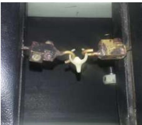
**Figure: 5** Flexibility of acetal resin clasp arm being tested in tensometer
