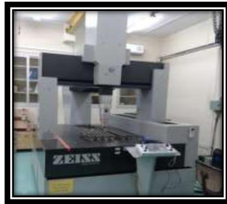
Fig 6. Co – ordinate measuring machine
