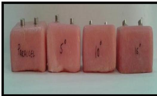
**Figure 1: Implant Analogues of Various Angulation (0°,50,100,150) Fixed In Resin Blocks**
